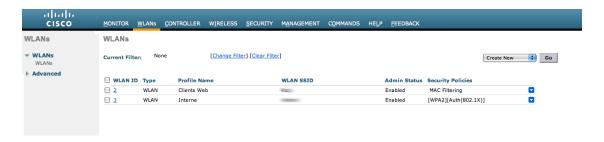
• In the secure SSID, make sure 802.1X is enabled and select the appropriate encryption for your needs (recommended: WPA + WPA2)
