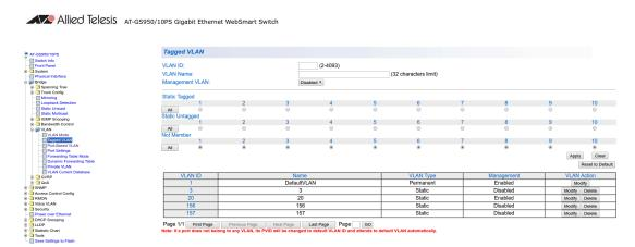
Note that they only need to be tagged on the trunk and don't need any specific configuration for the dynamic VLAN assignment here.
