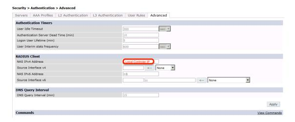
The next step will be to configure the Aruba WiFi controller for WebAuth in PacketFence, add the switch with the model choice **Aruba Network**,
