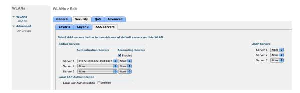
VERY IMPORTANT: Allow AAA override (this allows VLAN assignment from RADIUS)
